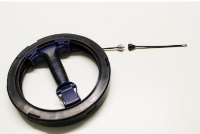
Fig. 14: Screwing the Push rod onto the viper
