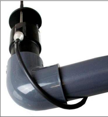
Fig. 31: Probe connected to the extension pipe.
