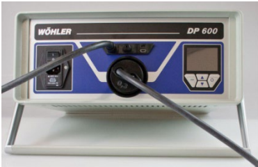
Fig. 23: Connection of the pressure tube and the air tube to the Wöhler DP 600
