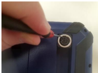
Fig. 10: Remove seal from the monitor connection
