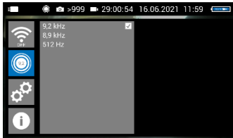
Fig. 29: Locator detection with 9,2 kHz transmission frequency selected
