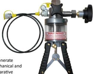
The Pressure Test Pump LR-Cal LPP 700 is used to generate pressure for checking, adjusting and calibrating mechanical and electronic pressure measuring instruments by comparative measurements. These pressure tests may be carried out in laboratories, workshops or directly on-site at the measuring point.
