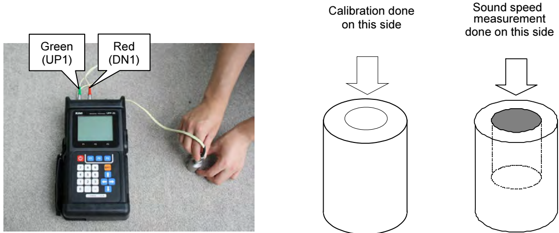
Fig. 1.2.4-9 Thickness and sound speed measurement
