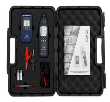
PCE-CL 10 is a wire tracer that uses the conductive method to detect metal pipes or pipe tracer wires. With PCE-CL 10, you also can locate power cables, lines, circuits, short circuits and ground points, as well as test protective tubing and coaxial cables. To perform these functions, it is not necessary to disconnect the power. Location can be identified in floors, ceilings, walls and the ground, even behind concrete and brick.
