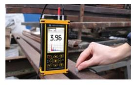
Ultrasonic thickness gauge is lightweight device, which will facilitate control both in difficult conditions in the field same as for production shops, special rubberized housings will protect against accidental drops.
