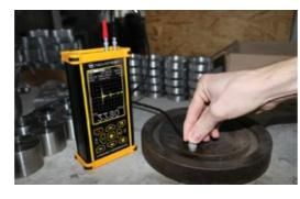
**A-scan** thickness gauge allows visualization of the signal for subsequent analysis by the operator. Making observation by screen of reflected signals it's able to eliminate false triggering, adjust the thickness gauges as correctly and accurately as possible.
