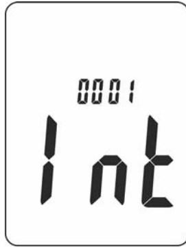
Fig. 7: Setting of the sampling interval
