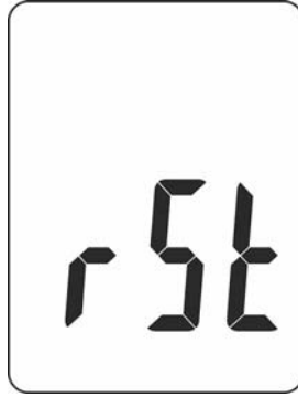
Fig. 5: Activating the instrument's reset
