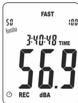
Fig. 8: Activation of SPL recording
