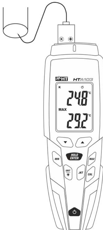
Fig. 5: Use of the instrument for temperature measurement
